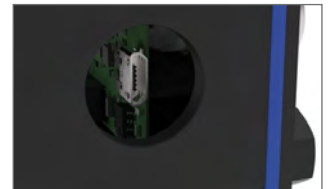
MICRO USB FOR PC CONFIGURATION
